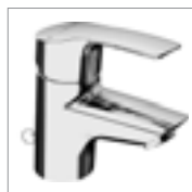
HANSAPOLO one-hole single-lever basin mixer, DN 15 5141 2273 chrome without pop-up waste, connection with flexible hoses G 3/8 projection: 90 mm
