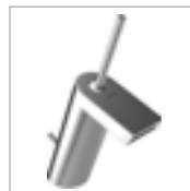
HANSASTELA one-hole single-lever basin mixer, DN 15 5709 2201 chrome pop-up waste (metal), connection with flexible hoses G 3/8 projection: 111 mm
