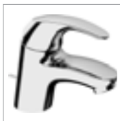
HANSAPICO one-hole single-lever basin mixer, DN 15 4604 2203 chrome pop-up waste (metal), connection with flexible hoses G 3/8 projection: 102 mm
