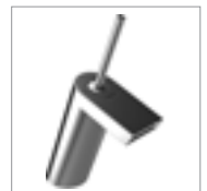
HANSASTELA one-hole single-lever basin mixer, DN 15 5713 1101 chrome # for open hot water heaters, pop-up waste (metal), connection using copper pipes projection: 111 mm
