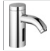
HANSADESIGNO-E electronic basin mixer, DN 15 battery-operated 5174 2210 chrome sensory operation (infrared), for cold or pre-tempered water only, without pop-up waste projection: 110 mm
