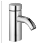
HANSADESIGNO-T self-closing fitting, DN 15, battery operated 5175 2211 chrome electronically controlled basin fitting with start/stop button, for cold or pre-tempered water only, without pop-up waste projection: 110 mm
